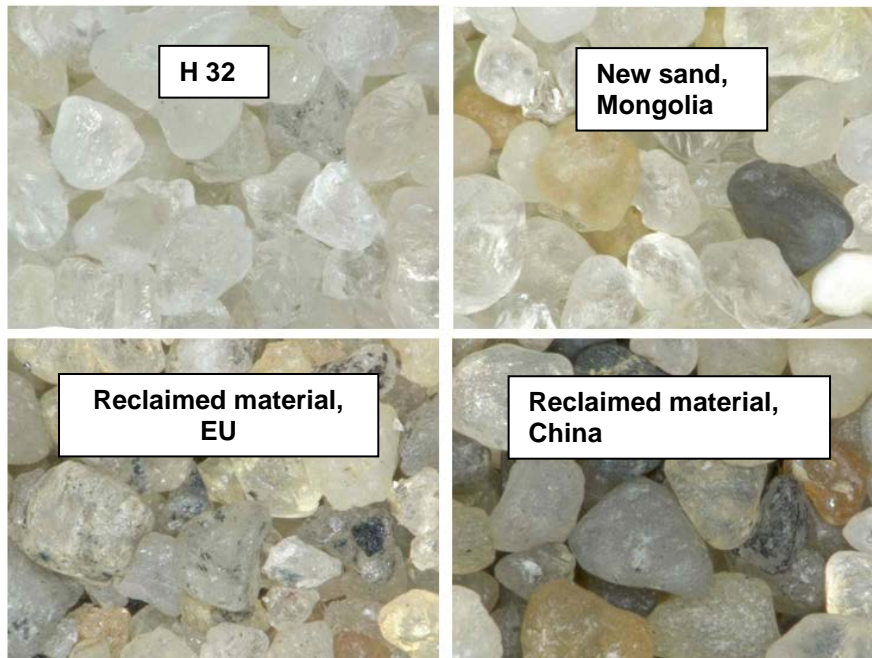
Fig. 8 Visual comparison of the sands at 200x magnification.
